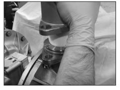
STEP 2 Remove the "Discharge Manifold".
