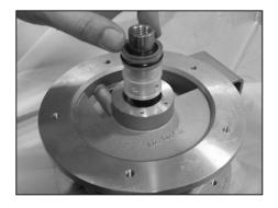
STEP 3 Remove the "Lip Seal" and "End Spacer".
