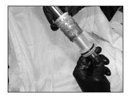
STEP 4 Remove "O-rings" and "Inner Spacer".
