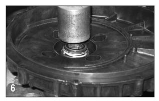
Remove carbon seal half from rear bracket with a round object. Tap gently with a hammer. Take care not to crack seal if reusing. Once disassembled; clean all reusable parts thoroughly, removing any traces of old gasket material and trapped / dried liquids from pump.
