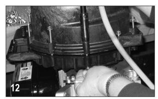
Install the pump body (12712/13712) as shown below with the outlet flange facing up. Install the 10 body screws (12720), 10 lock washers (V07018), and 10 nuts (V07019) to secure the pump body to the rear bracket. Tighten the bolts securely to 75-100 in lbs all the way around.
