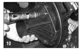
Install volute (12702A/13702) onto rear bracket using the three volute screws (12900/12725). Tighten the 3 screws to 8-12 in lbs. Install check valve (12705) onto the snout of the volute. Drive unit should be turned over a few times to check for clearance between the two. A small amount of drag between impeller and volute is ok, however, if the drive unit will not turn over because of the lack of clearance, a bracket shim may have to be used.
