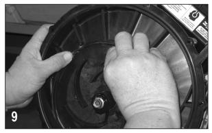
Install the O-ring segment (12754) onto the rear bracket as shown.
