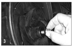
Remove the impeller bolt (12765A) from the impeller (12771A/12772). Remove the impeller bolt gasket (12774VA) from the impeller.
