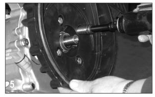
Remove the four bracket screws (12715A), rear bracket washers (12901), and screw head O-rings (12717) from the rear bracket using a ½" socket. With the four bracket screws removed, the rear bracket can now be removed from the drive unit.
