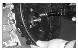
Install the rear bracket onto the drive unit using the bracket screw assemblies from the previous step. The handle of the rear bracket should be to the top of the drive unit. Tighten the screws securely to 125-150 in lbs.
