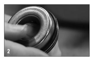
Place the seal O-ring (12710) behind the lip of the carbon seal half.
