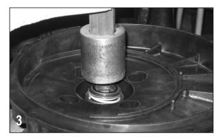
To install the carbon seal (12713) half into the rear bracket use a tool such as a 2" hose barb or arbor press to give even pressure on the metal flange of the seal housing during installation.
