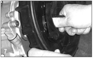
Place the impeller key (12902A) in the slot located inside the impeller snout. The impeller (12771A/12772/13772) is now ready to be slid onto the drive unit shaft. Be sure to align key with the keyway of the drive unit shaft.
