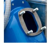
Large inspection covers Easy access to float box, impeller and non-return valve.
