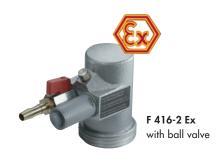
**Air motor**, explosion-proof to II 2 G c IIC T6, easily variable speed control by adjusting either the air supply pressure or volume, motor overload-proof, air connection G 1/4 (BSP 1/4" female).
