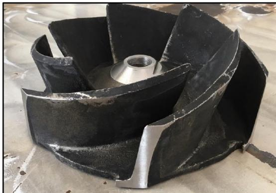
*Condition of new impeller, before grit blast.*
