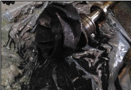
*Catalyst built up in the Impeller: needle gun cleaning was required.*
