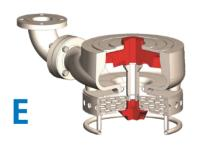
The **E Wet End** has a fully recessed vortex impeller that permits an unobstructed passage of large solids. Fibrous material can also be handled without difficulty due to the natural flow of the fluid through the pump casing and the fact that the flow is virtually isolated from the impeller (only 15% of pumped liquid is in contact with the impeller). This pump is ideally suited for low shear applications.
