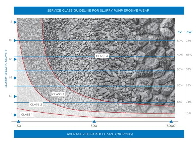
The above chart is for use as a guide only. It assumes 2.65 Ss silica-based solids. Adjust rating to account for solids of different abrasivity using ASTM G75-95. The chart is based on the Hydraulic Institute's Slurry Class guideline. For more information about the HI Slurry Classes please visit http://pumps.org or call HEVVY PUMPS for assistance.
