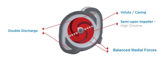
With the **Twin-Volute** design, the thrust force is balanced by **opposing 180 degree discharge outlets**. The result is less loading on the motor bearings and seal which will extend the life of the pump.
